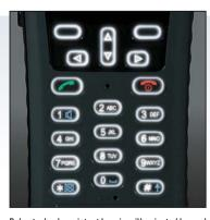
Robust, shock-resistant housing, illuminated keypad with good differentiation for use when wearing gloves
